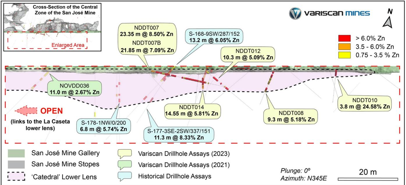
**Figure 2. 3D model illustrating newly defined La Catedral Lower Lens, Central Zone, San Jose Mine**
