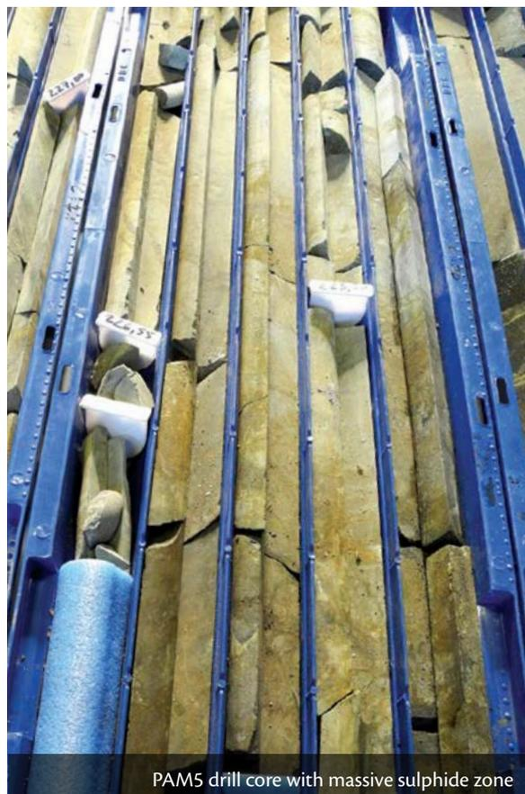
PAM5 drill core with massive sulphide zone
