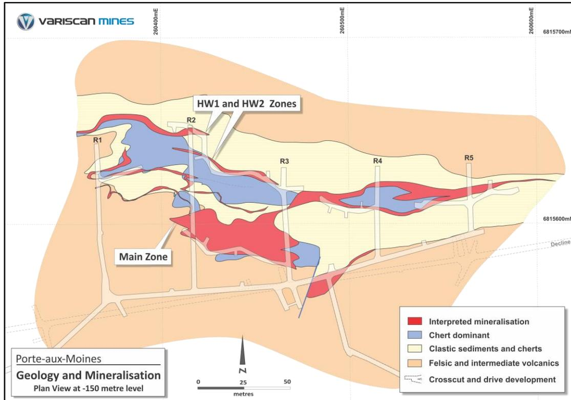
**Figure 3: Plan view of Porte-aux-Moines deposit showing interpreted mineralised zones and underground development completed by the BRGM**
