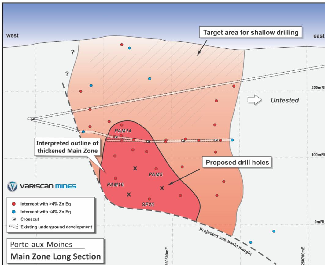
**Figure 2: Vertical long section of the Main Zone surface at PAM showing the interpreted thickened zone and flanking mineralisation. Proposed deeper drilling pierce points shown as well as the target area for shallow drilling (hatched)**
