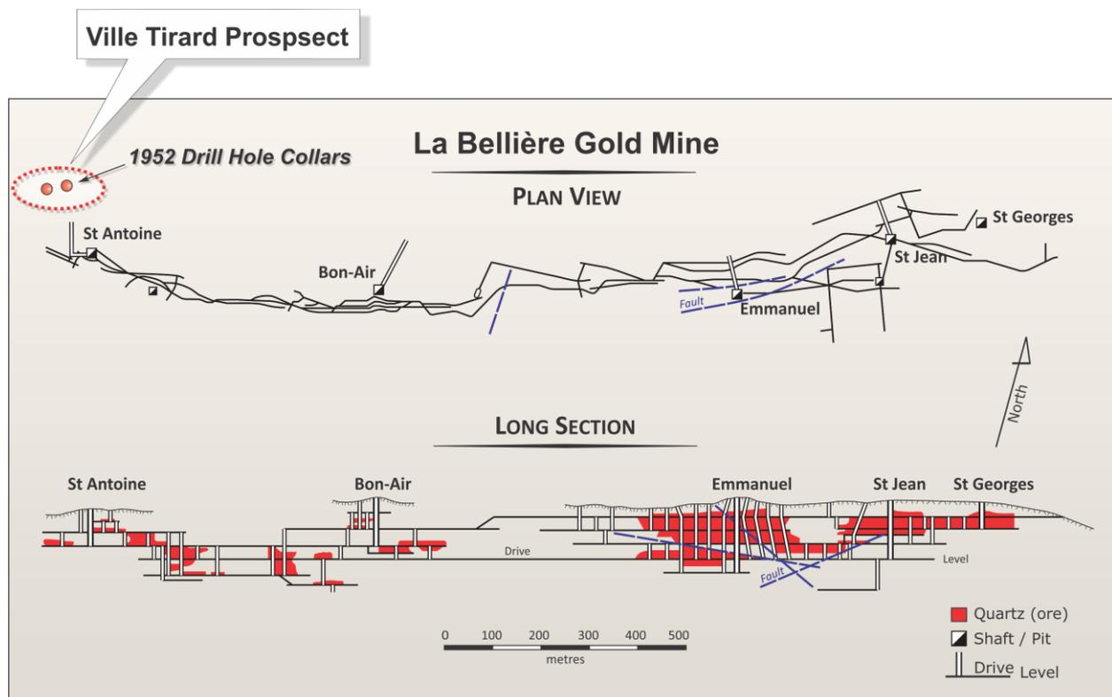
**Figure 7: Approximate location of Ville Tirard prospect and drill collars from 1952 drilling projected onto the plan view of the La Bellière gold mine workings**
