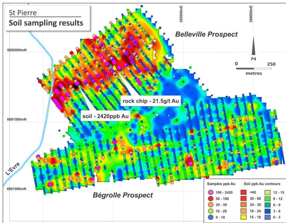
**Figure 6: Belleville gold prospect at St Pierre showing soil sampling completed to date and strong anomalism defined**
