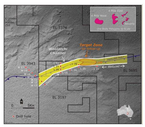
Figure 3 - Greyscale topographic image showing interpreted Woolatchi channel - oxidised palaeochannel sands discovered within Namba Formation shale sequences. W-series are historic drill holes. L-series are Red Metal holes. Small gamma anomaly in hole L26 suggests potential for uranium roll-front further east down the channel.
