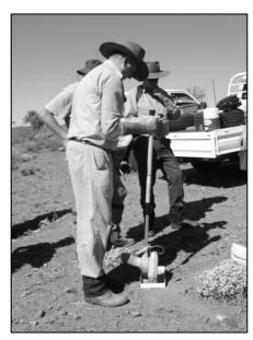
Using the Niton portable XRF analyser at Broken Hill
