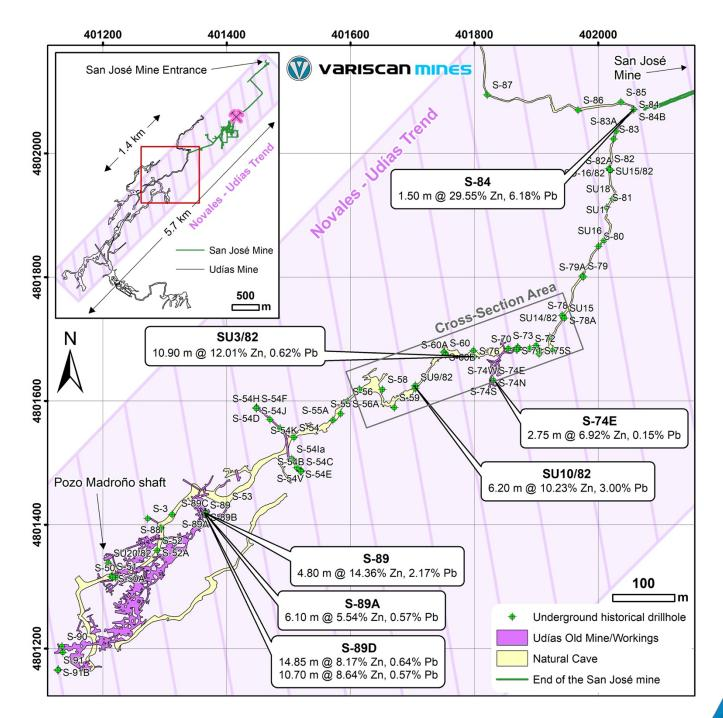
**Figure 1.** Plan view of drill-hole data illustrating significant exploration potential as mineralisation extends on strike to the south west of San Jose Mine
