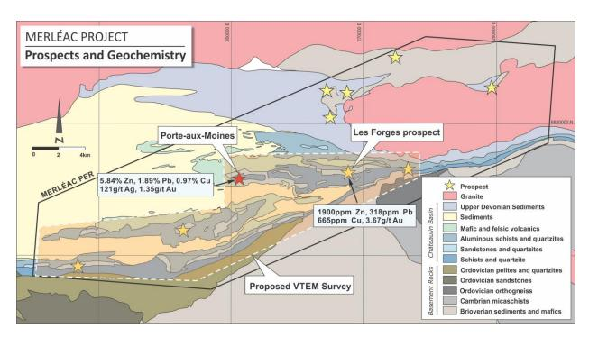
Figure 4 – Peak ALS assays in sampling at Porte-aux-Moines and the Les Forges prospect
