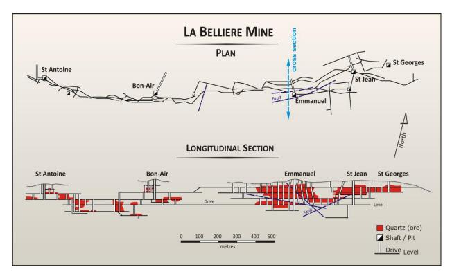
Figure 5 – Plan and long section views of La Bellière mine
