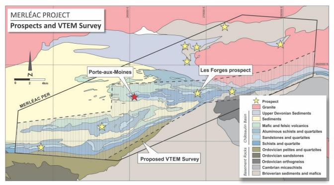
Figure 1: Key VMS prospects and outline of the VTEM survey at Merléac
