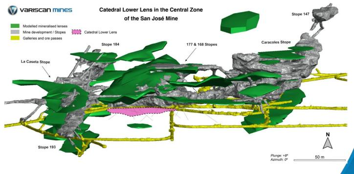
**Figure 3.** Plan view of drill-hole data illustrating newly defined La Catedral Lower Lens, Central Zone, San Jose Mine
