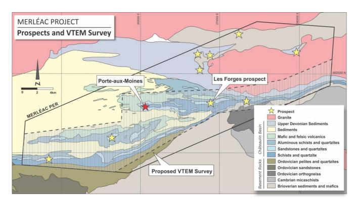
Figure 4: Key VMS prospects and outline of the VTEM survey at Merléac
