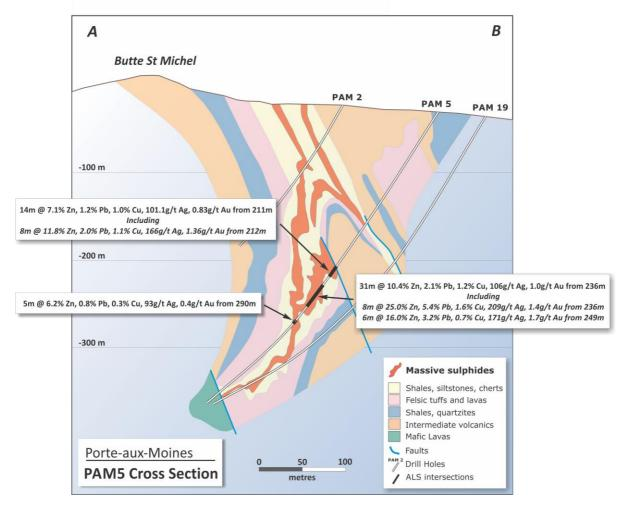
Figure 3 - Cross section through the Porte-aux-Moines deposit highlighting the ALS assays in PAM5. The geological interpretation comes from BRGM reports.
