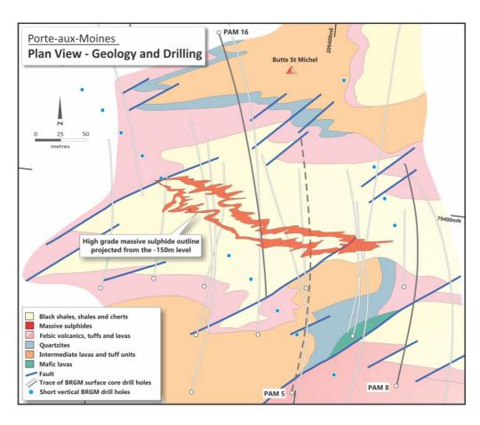
Figure 2 – Plan view of the surface geology at Porte-aux-Moines and BRGM core drilling showing the location of PAM5 and the approximate projected position of the high grade massive sulphide zones 150 metres below the surface as interpreted by the BRGM.
