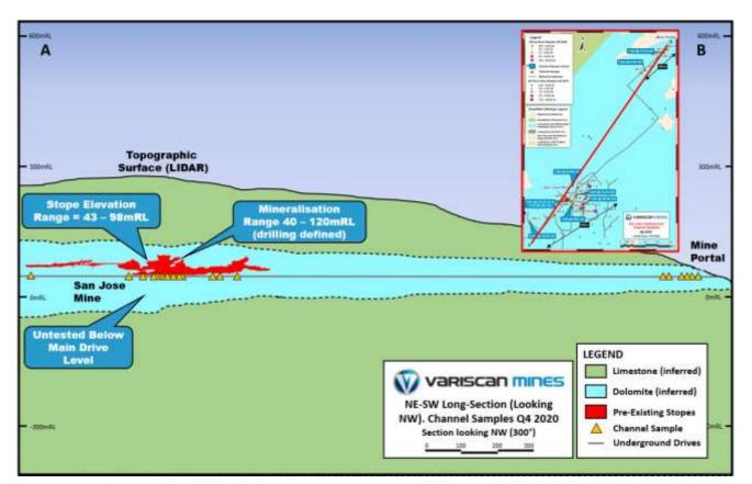
As shown in Figure 2 and Figure 3, the mined-out stopes range in elevation between +43m to +98m, as demonstrated by the 3D underground laser survey completed in 2020. However, the historical drilling indicates this typically stratabound mineralisation ranges between +40m and +120m elevation, providing significant upside for exploration at unmined levels.
