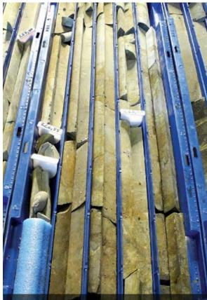
PAM5 drill core with massive sulphide zone
