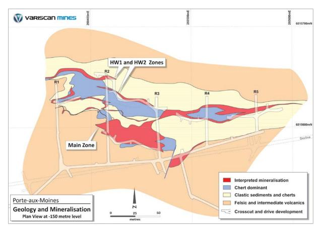
Plan view of Porte-aux-Moines deposit showing interpreted mineralised zones and underground development completed by the BRGM
