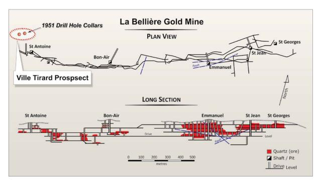
Approximate location of Ville Tirard prospect and drill collars from 1952 drilling projected onto the plan view of La Bellière gold mine workings
