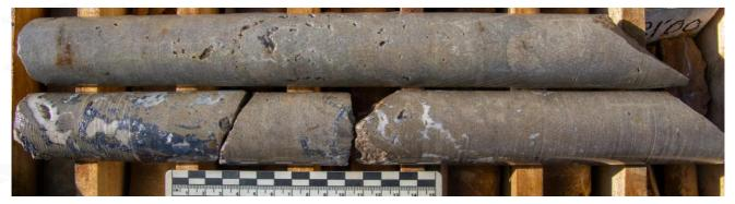
Drillhole NOVDDT005, interval shown 1.05 – 1.80 m: high-grade replacement-type zinc ore
