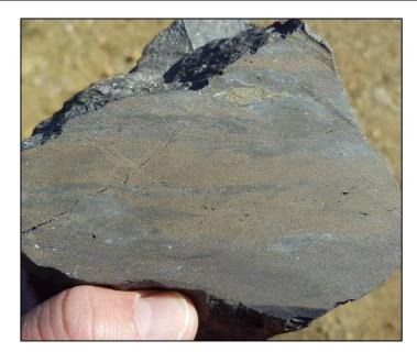
Figure 10:High-grade massive sulphide mineralisation dominated by sphalerite (pale brown).From BRGM waste dump at Porte-aux-Moines prospect.
