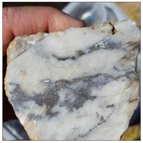
Figure 19:Sample of orogenic gold mineralisation from La Bellière Gold Mine.Quartz-arsenopyrite-pyrite-sphalerite vein held by CSA Global geologist, Thomas Branch.
