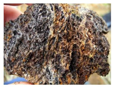
Figure 14: Massive spongy gossan texture after pyritic sulphide mineralisation. Notre Dame Iron Workings in far south-east of project (Maund, 2014a)
