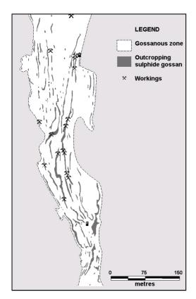
Geological map of Yalcowinna Creek prospect, Euriowie Project, NSW. Wide gossanous zone extends over a 700 metre strike length. Anomalous rock-chip values up to 2.2 g/t gold, 100 g/t silver and 12% copper. No previous drilling
