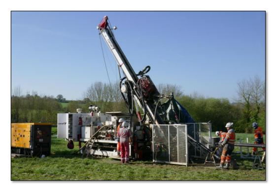
Plate – RC drill rig at Belleville, April 2017
