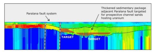
Figure 4 - Lakes Project: REPTEM inversion section showing the interpreted thickened sedimentary package adjacent to the Paralana fault which is being targeted for prospective channels sand facies hosting uranium. The deep penetrating Paralana fault may also control the upward flow of uranium enriched basement fluids into the prospective sands units.
