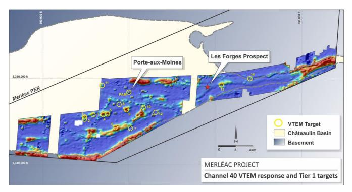
Figure 1: 'Tier 1' VMS targets over Channel 40 response plot at Merléac
