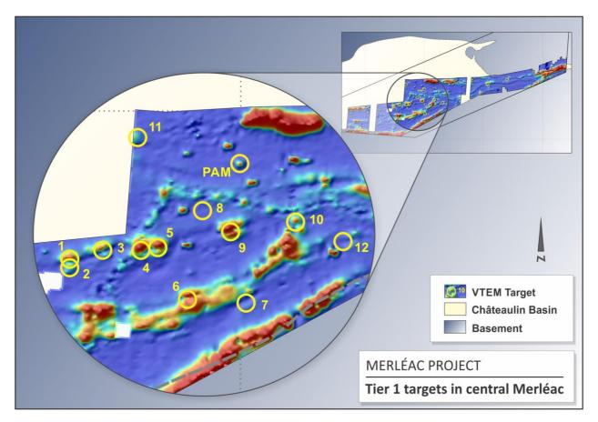
Figure 2: 'Tier 1' VMS targets over Channel 40 response plot in the centre of Merléac licence around the Porte-aux-Moines VMS deposit (PAM). Targets defined principally by anomalous early to mid-time responses (e.g. target 8) will appear subdued on this late-time image.
