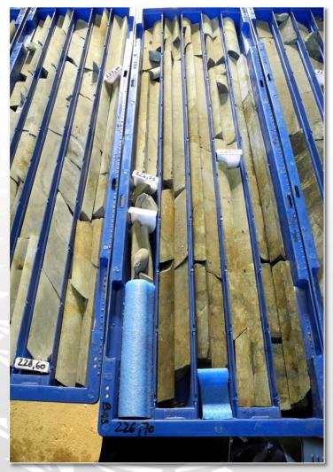
Massive sulfide zone in PAM5
