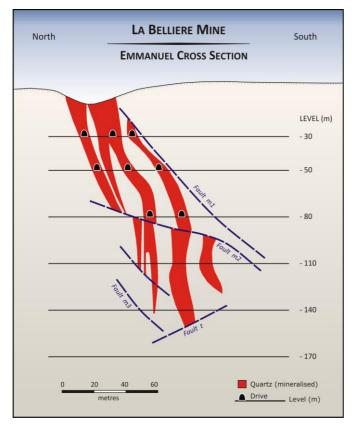
Figure 3 – Cross section through Emmanuel - La Bellière mine
