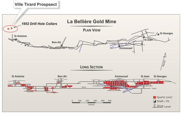
Figure 5: Approximate location of Ville Tirard prospect and drill collars from 1952 drilling projected onto the plan view of the La Bellière gold mine workings
