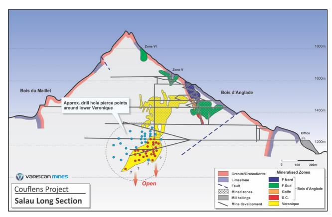
Figure 3 - Composite long section through the Salau mineralised system showing the key mineralised zones defined from previous exploration/mining. Approximate recorded position of LMA underground drilling testing the lower section of Veronique shown in yellow (red - >1.0% WO<sub>3</sub>, blue - low grade/barren). Source - Dr. Nick Le Boutilliere.
