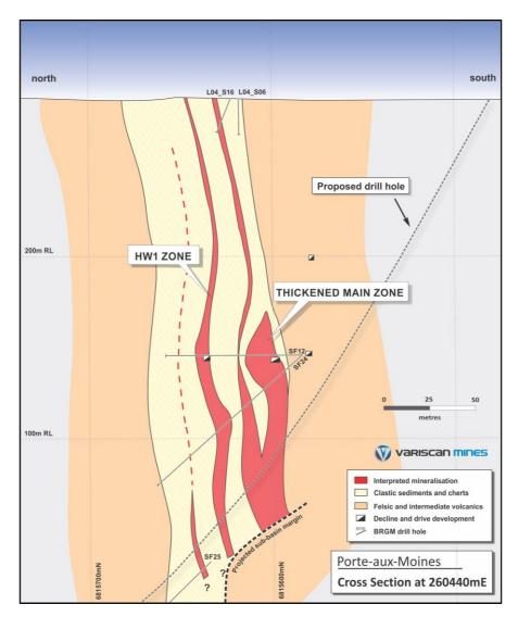
Figure 7: Cross section at PAM showing interpreted mineralised zones and proposed future drilling
