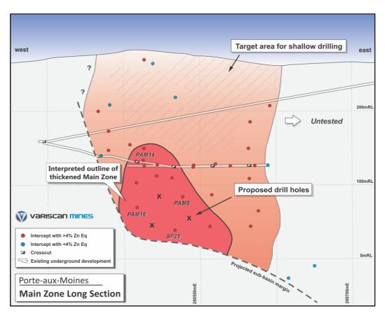
Figure 6: Vertical long section of the Main Zone surface showing the interpreted thickened zone, flanking mineralisation and proposed deeper drilling
