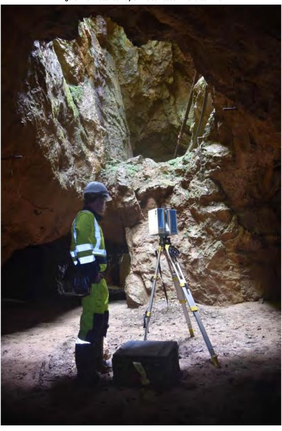
Figure 4. 3D Laser survey of the San Jose - Novales Mine
