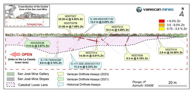
Figure 5. 3D model illustrating newly defined La Catedral Lower Lens, Central Zone, San Jose Mine
